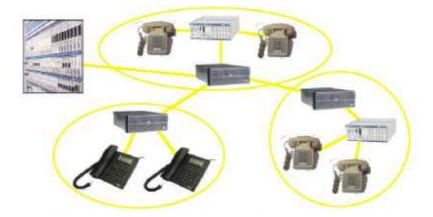
One of iPBX most powerful features is its ability to link remote offices of a SME (Small to Medium Enterprise) together. The above diagram shows how you can build individual small PBXs for multiple offices using iPBX, and then link them together transparently into a single network.
